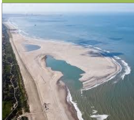
Sand motor' beach replenishment, Ter Heijde, Netherlands
