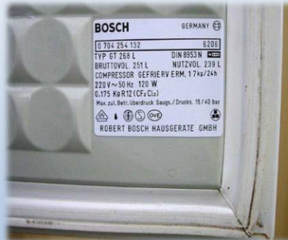
Refrigerator with prohibited refrigerant: R12 – no second hand product, no Green List waste - HAZARDOUS WASTE
