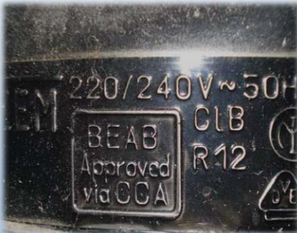
Old compressor containing CFC: R12 – no second hand product, no Green List– HAZARDOUS WASTE
