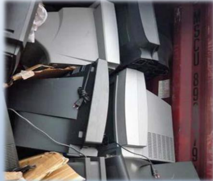
Monitors without packaging, inadequately stored during transport - HAZARDOUS WASTE
