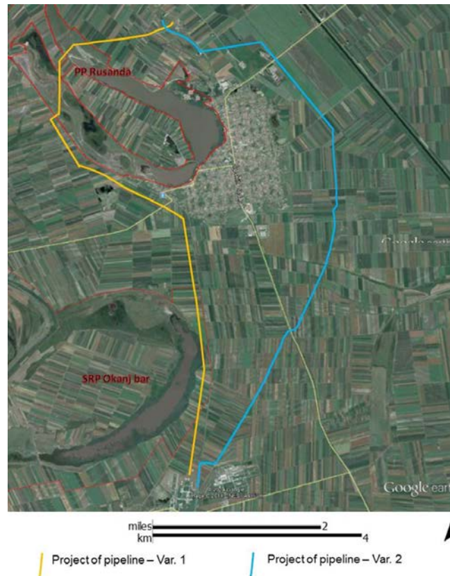
Fig. 3 Two alternative variants of the pipeline for CO 2 between the CO 2 separation unit in Elemir and old wells in Melenci
